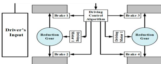
**Figure 3.** Main working components of the driving control system for four-wheel-drive EVs proposed by Juyong Kang et al. The driving control algorithm takes the driver's inputs, and then determines the actions of the brakes and the motors according to the control mode [25].
