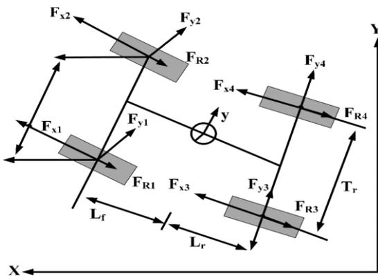
**Figure 2.** Forces acting on the wheels of a car. Each of the wheels experience forces in all three directions, marked with the ‘F’ vectors.  $L_f$  and  $L_r$  show the distances of front and rear axles from the center of the vehicle, while  $T_r$  shows the distance between the wheels of an axle. Adapted from [8].
