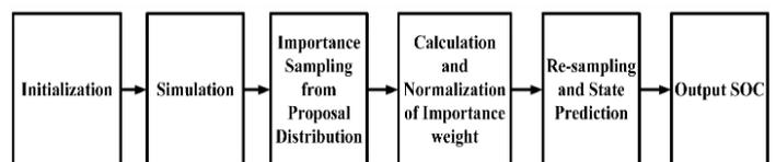
**Figure 5.** Working principle of the SOC measuring algorithm proposed by Zhou et al. [180].
