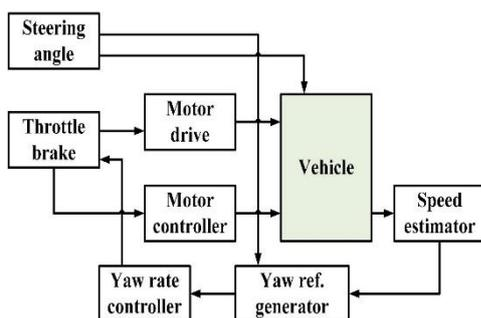
**Figure 4.** Working principle of vehicle stability system proposed by Tahami et al. A neural network was used in the yaw reference generator [8].
